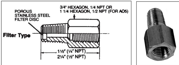
**Filter Type:** Snubbing element consists of a  $\frac{3}{8}$ " diameter x  $\frac{1}{8}$ " thick Micro Metallic stainless steel filter. When placed in the line just before the pressure gauge, the gauge pointer moves across the scale at a rate which is proportional to the pressure differential across the snubber element.
