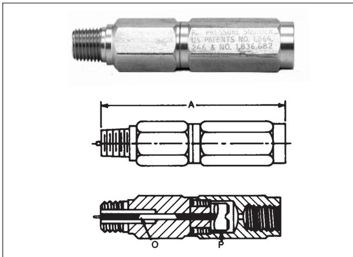
**Piston Type:** Shocks and pulsations are absorbed in the doughnut-shaped orifice (O) formed by the piston (P) in the tube. As the piston moves up and down with the pulsation, it automatically clears away any sediment or pipe scale that would clog a simple orifice or needle valve.
