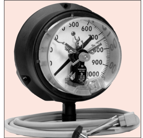
Indicating accuracy of Royal Gauge, above 300 psi with contact: Pointer not carrying contact – 1.0%. Pointer carrying contact – 1.5%. For ranges below 30 psi, add an additional ½% to indicating accuracies.
